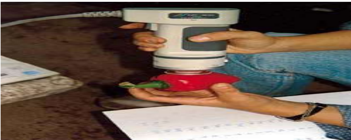
Fig. Objective colour measurement with a colourimeter
