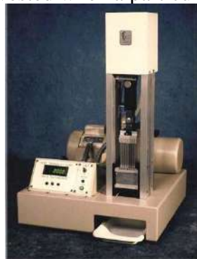
Fig. Tenderometer to test the pea maturity by presser tester
