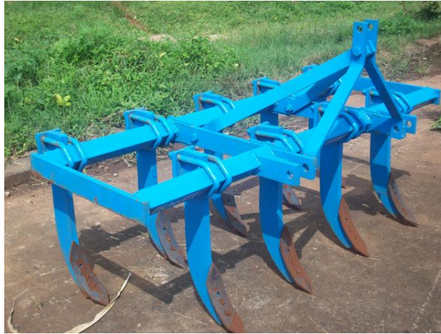
Plate : 15.2 Rigid tyne cultivator
