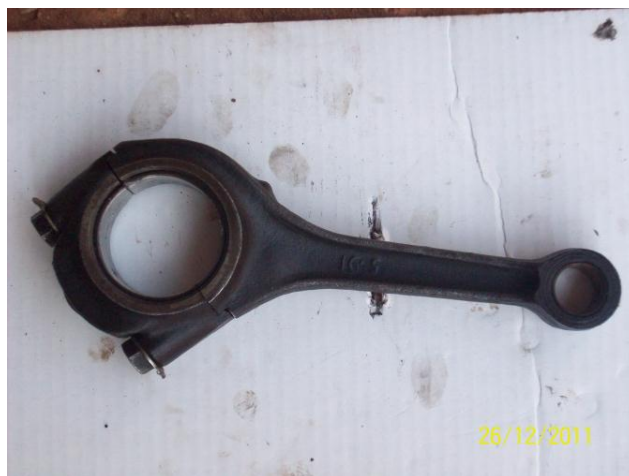
Plate : 2.8 Connecting rod
