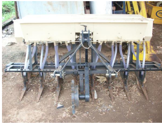
Plate : 16.1 Tractor drawn Seed cum fertilizer drill
