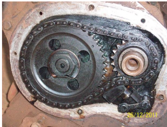
Plate : 2.13 A view of timing gear and chain arrangement
