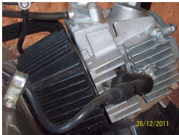
Plate : 5.1 A view of fins provided on the cylinder
